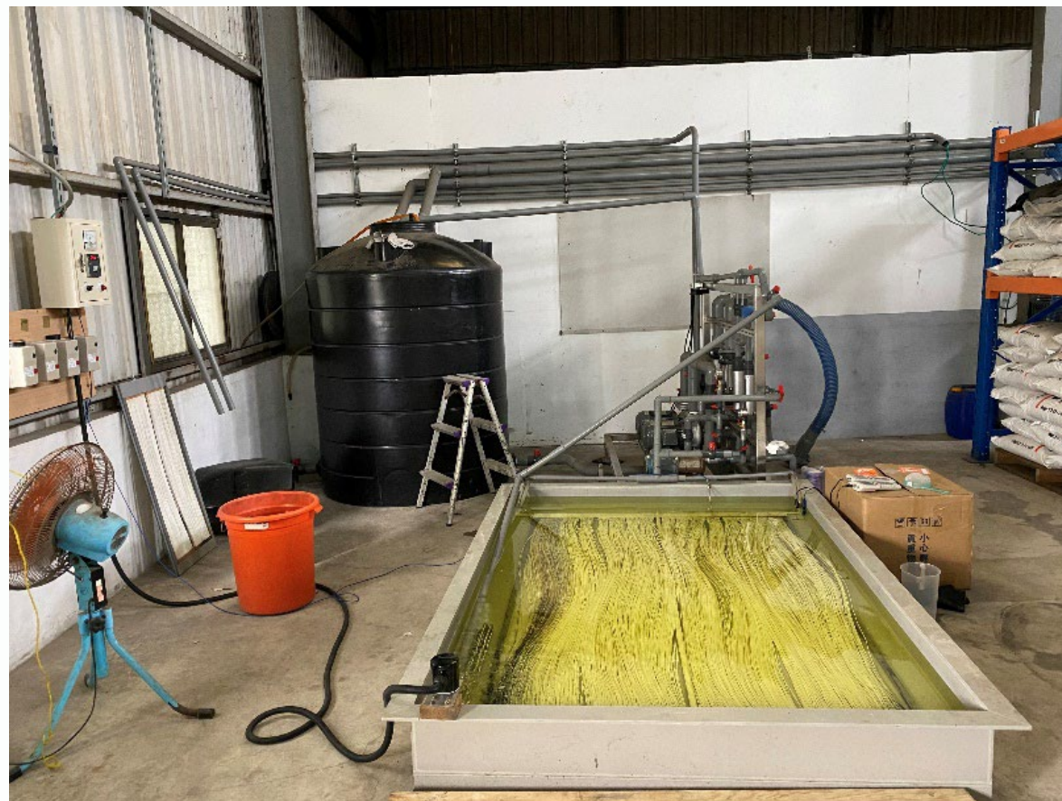
SMF membrane chemical cleaning test experimental device
