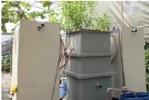
Fig. 1: Pilot-scale bioretention unit to assess the impact of filter media depth and plants on effluent water quality
